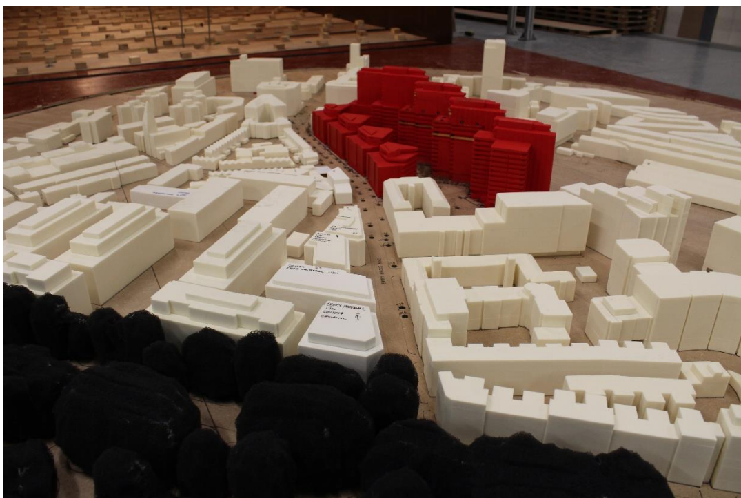
Figure 8: Photo of the masterplan model in the wind tunnel in future surroundings (view from the south-west)
