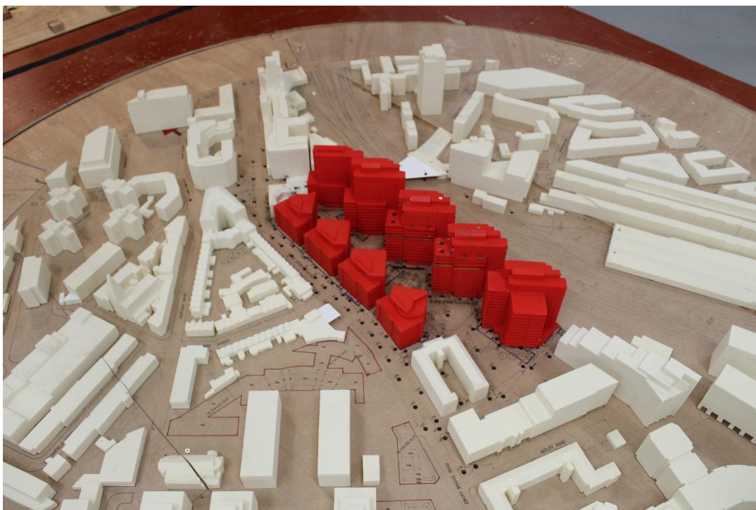
Figure 6: Photo of the masterplan model in the wind tunnel in existing surroundings (view from the south-west)
