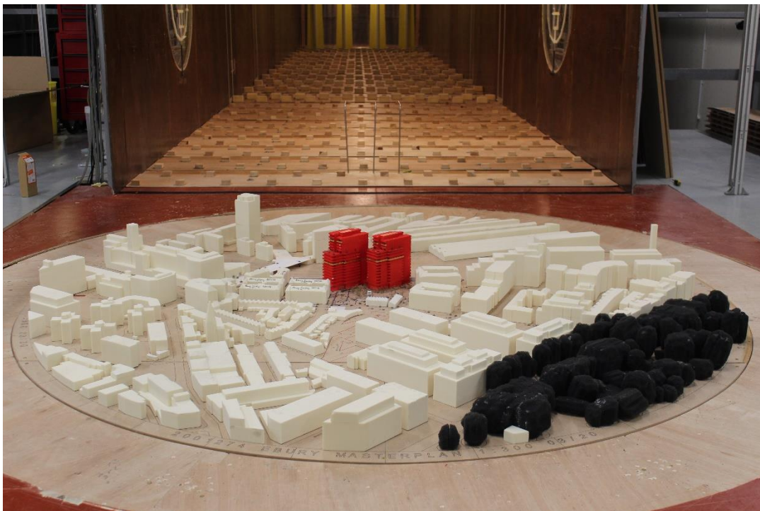
Figure 4: Photo of the Detailed Area model and existing surroundings in the wind tunnel (view from the west)
