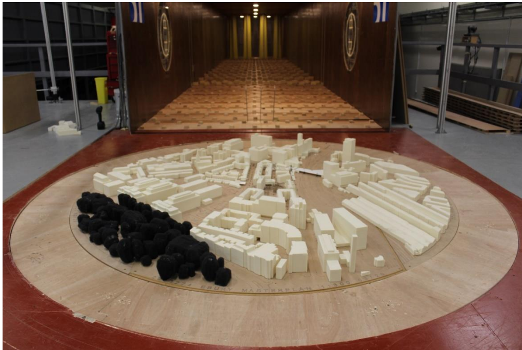
Figure 1: Photo of the model in the wind tunnel for the existing scenario (view from south)
