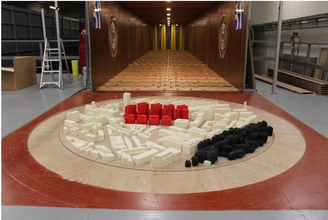
Figure 5: Photo of the masterplan model in the wind tunnel in existing surroundings (view from the west)
