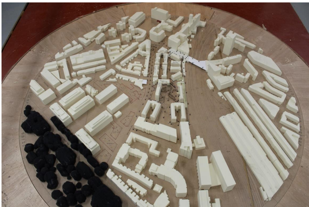
Figure 2: Close up photo of the model in the wind tunnel for the existing scenario (view from south)
