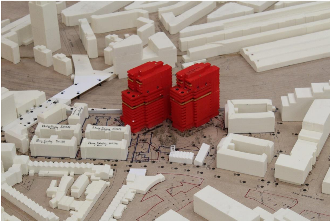
Figure 3: Photo of the Detailed Area model in the wind tunnel (view from the west)
