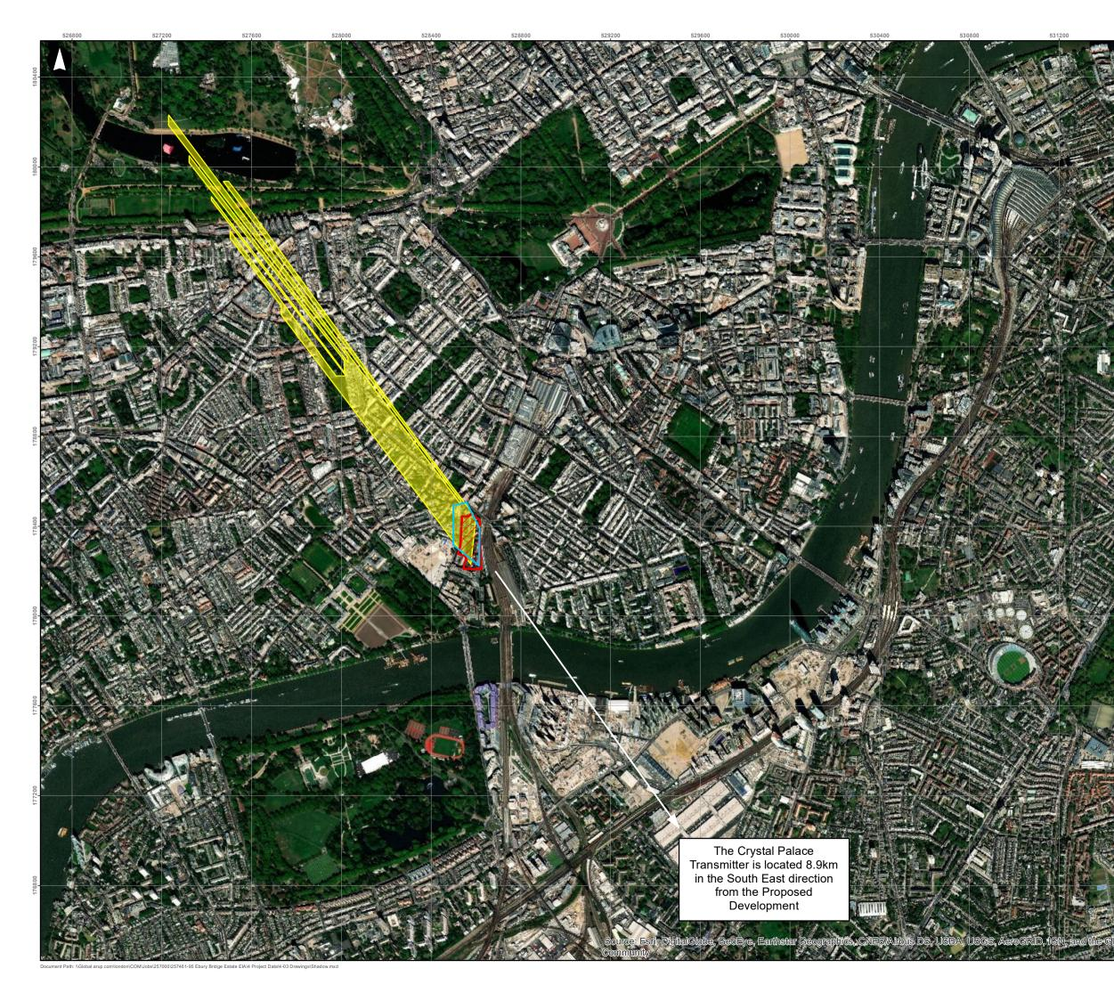
Notes 1. To be read in conjunction with Ebury Bridge Renewal Environmental Statement Electromagnetic Interference (EMI) topic chapter Legend Proposed Development Site /// Astra Satellite Signal Shadow Crystal Palace Transmitter Signal Shadow
